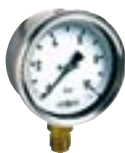
Radial - Ø 100 Class 1,6 - Connection 1/2" - TS: +180°C - To be installed with coil siphon.
