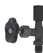
Pressure gauge valve DIN 16270 A type - Carbon steel body - M1/2" x F1/2" - PS: 400 bar - TS: +200°C.
